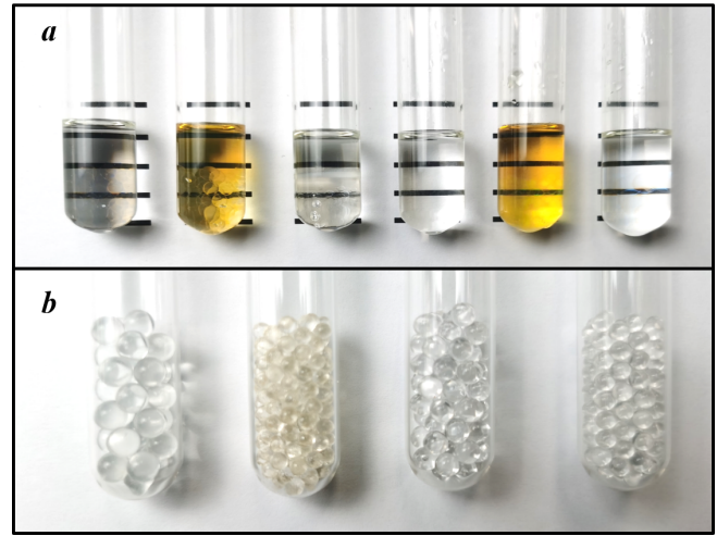
Fig. 4. (a) The mixture picture of particles and liquid, left to right: 87.25% tetralin-ethanol solution and H-K9 glass, 12.4% engine oil-benzene solution and organic glass, p-cymene and organic glass, water and super absorbent resin, 59% NaI solution and high borosilicate glass, 59% NaI solution and high borosilicate glass with \text{Na}_2\text{S}_2\text{O}_3 as a decolorizer; (b) The picture of particles, left to right: H-K9 glass, organic glass, high borosilicate glass, super-absorbent resin.
